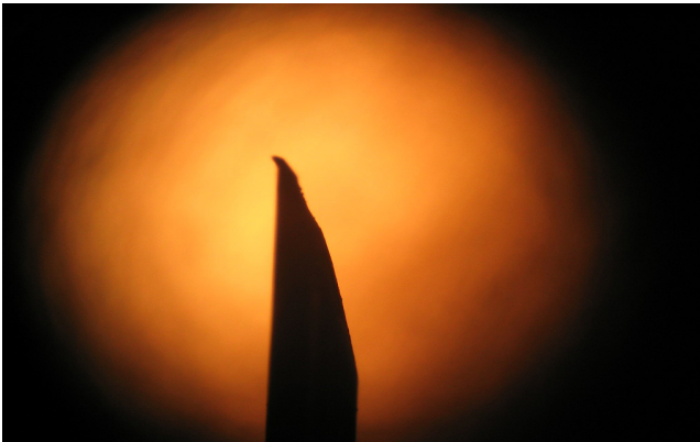
Photo 22: New needle from box, not good enough
