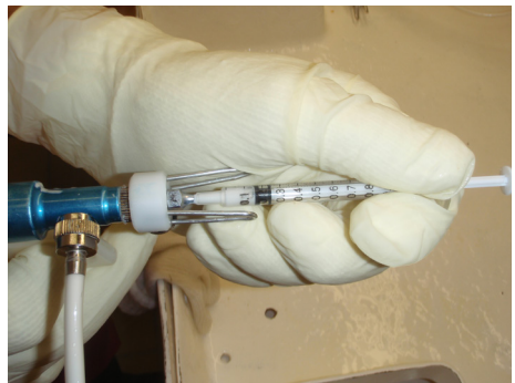
Photo 6: Calibration using 1 ml syringe
